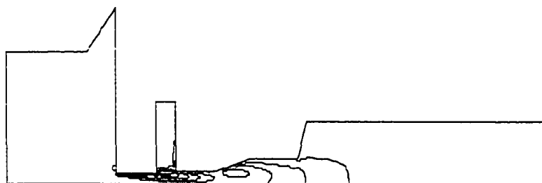
Figure D.2 Turbulent Kinetic Energy Contour for Pulsed Nozzle (Contour Level: k_{\max} = 0.249 \times 10^9 \text{ cm}^2/\text{s}^2 and k_{\min} = 0.160 \times 10^4 \text{ cm}^2/\text{s}^2 ) at t = 0.5 \times 10^{-3} sec After Initiation of the Pulsate Flow; (Test conditions are identical to those in Fig. D.1).
